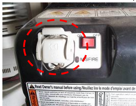
Picture 5 Inspection terminals for control device(PH1)
