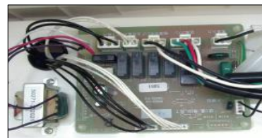
Actual installation of circuit board on RKF unit Note the circuit board is up side down from the left picture
