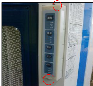
Remove 2 circled screws Pull out the entire indicator plate assembly
