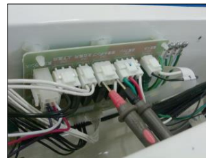
Picture 4: How to measure voltage
