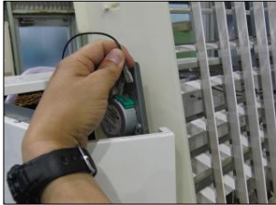
When vertical louver motor appears by pushing up the entire louver guard, detach lead wires from the louver motor. Then, remove the entire louver guard assembly.
